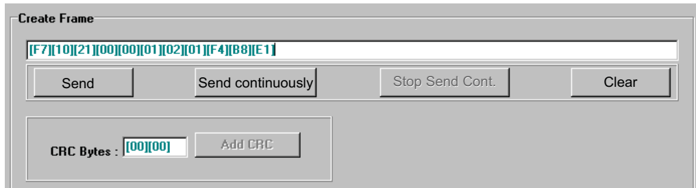
Figure 8: Frame sent to the Modbus-Module
